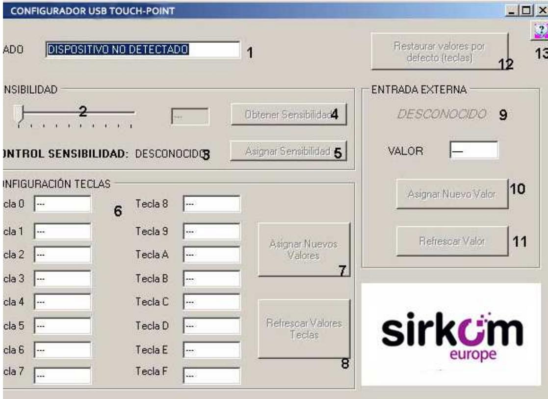
The status indicator is shown in the upper part (1). When the device is not connected, as shown in this example, “DEVICE NOT DETECTED” will be displayed and all other controls will be deactivated.
